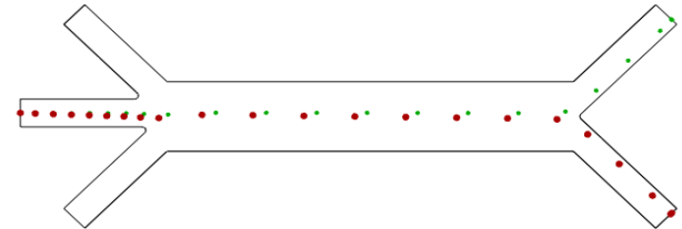
Fig. 11. The particles are emitted simultaneously and in the same direction. RBCs are shown in green, while cancer cells are shown in red.
