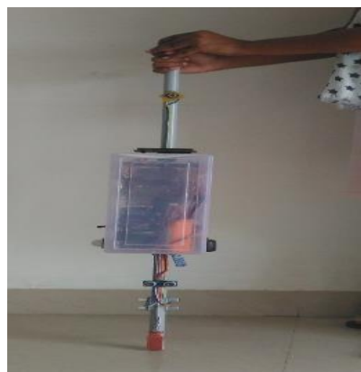
Fig. 4 complete intelligent walking stick
