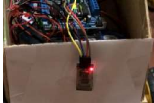
Fig. 7. Pin connections with Bluetooth module of the remote control robot.
