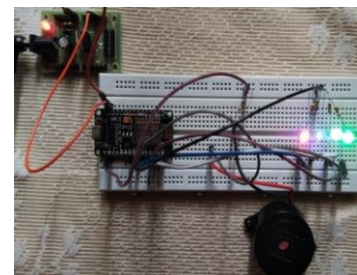
Figure 5: Simulation of Voice controlled home automation system with all light and buzzer ON
