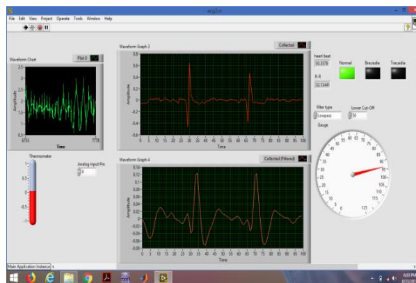
Fig.9: The front panel of LabVIEW for the detection of Heart Rate.
